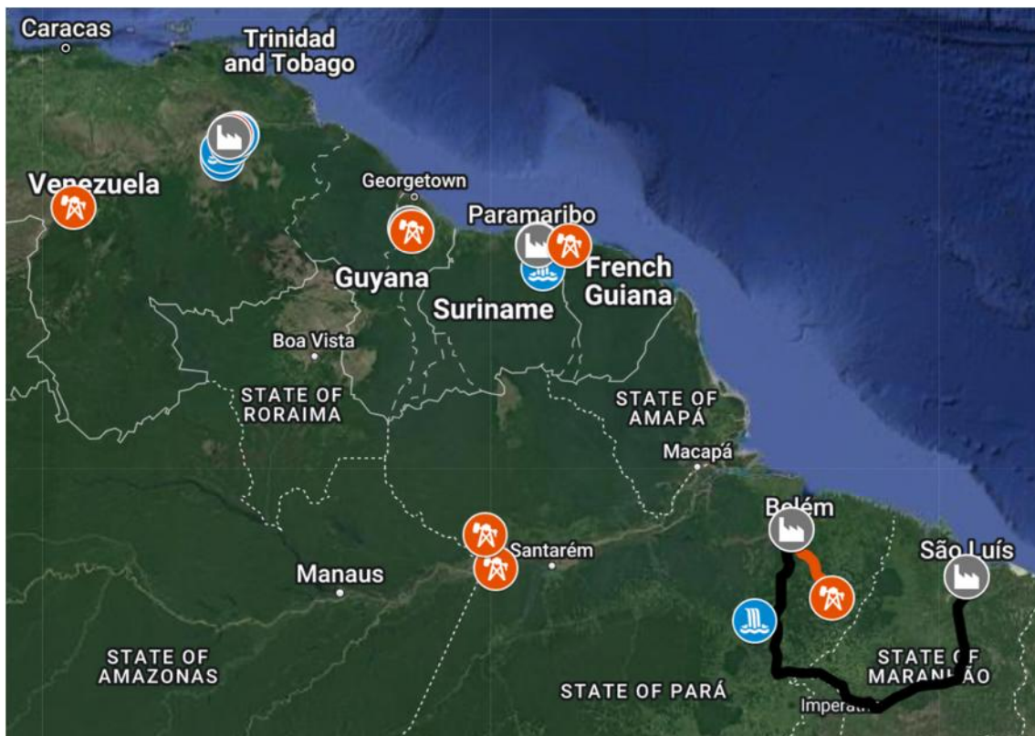
Figure 1. The northeastern Amazon, with the different components of the aluminium supply chain. The orange symbols indicate bauxite mines, grey symbols alumina–aluminium production facilities, and the blue symbols major hydroelectric plants. The black lines indicate the main electricity transmission lines connecting the hydroelectric plants to the aluminium plants, while the red line shows the slurry pipeline transporting liquefied bauxite from Paragominas to the alumina plant in Barcarena. Source: Own elaboration using Google Maps.
